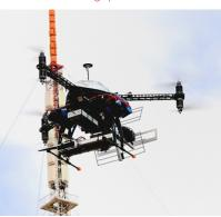
The UAV with the measurement payload
