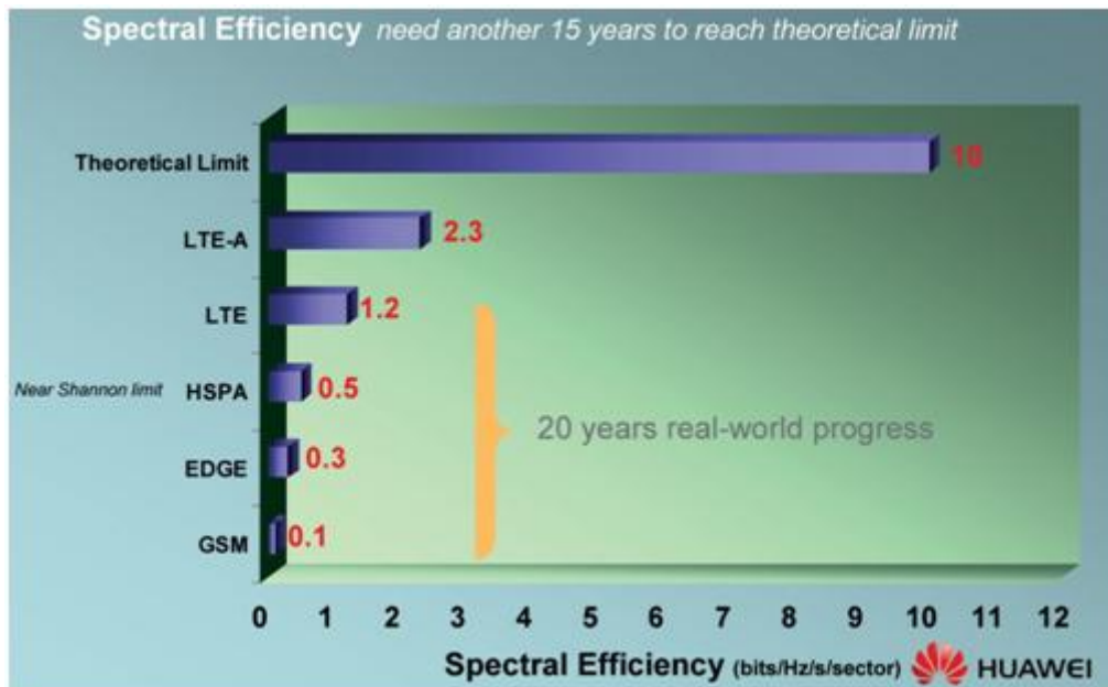
Figure 3-1: Huawei forecasts of spectrum efficiency of IMT technologies [Source: ‘LTE-A and Beyond’, Huawei, Latin American Spectrum Conference 2013]
